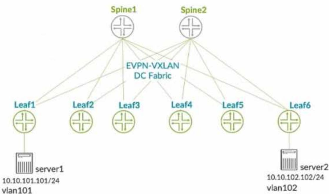
You connect two single-homed servers using Juniper Apstra as shown in the exhibit. You are using the ERB design blueprint with two virtual networks in a common routing zone.
